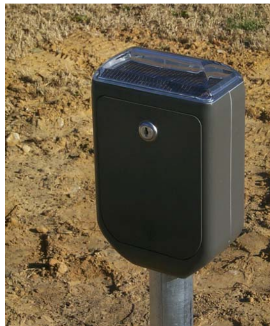
Solar-powered irrigation controller
